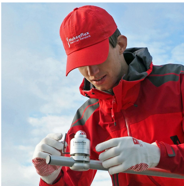
Figure 2 Easy levelling of SR05 on its tube mount with ball levelling. SR05 series offers various industry standard digital and analogue outputs.
